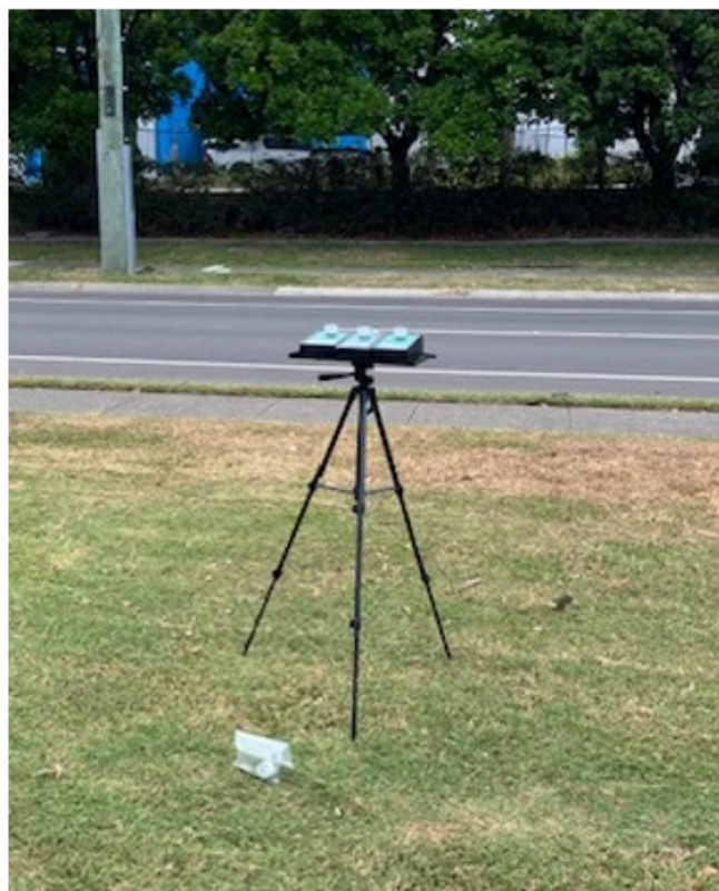
Figure 1 Sampling setup for collection of 3 samples simultaneously using 3 Bio-pump air samplers.
