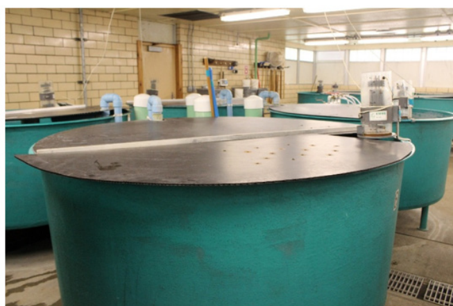
Figure 2 Photograph of a tank near-completely covered with a non-submerged structure made of corrugated plastic.
