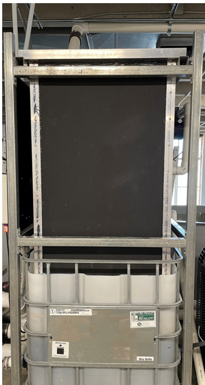
Figure 11 Front of degassing tower with the intermediate bulk container used as collection vessel.
