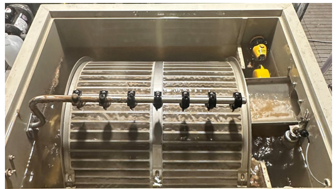
Figure 6 Drum filter with 70-micron screen.
