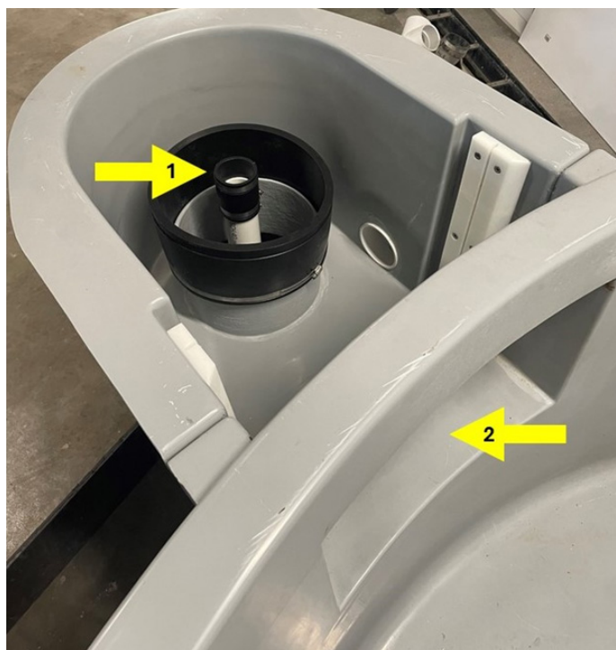
Figure 2 Effluent point from the central drain (1), and remaining tank effluent route (2).
