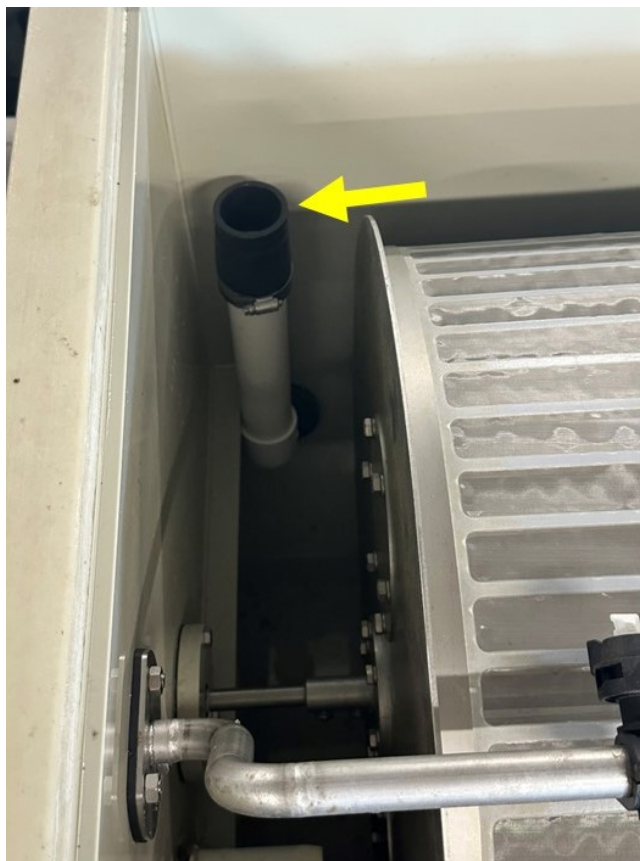
Figure 16 Standpipe governing maximum water level on the treated effluent side of the drum filter.
