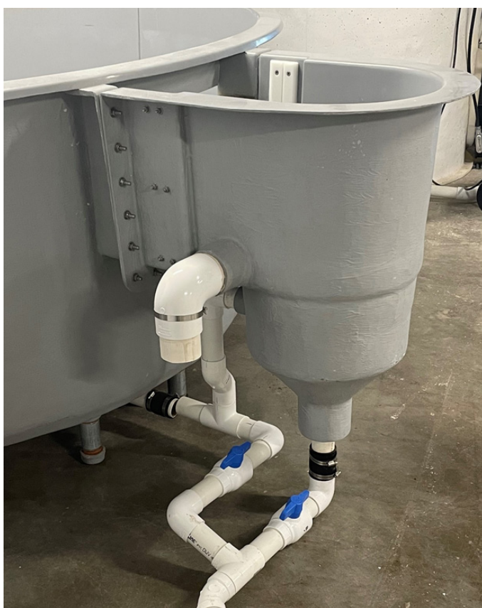
Figure 1 Radial flow settler (RFS) bolted to the side of the culture tank.
