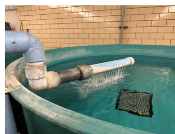
Figure 1 Image of a circular tank with an elevated horizontal spray bar.
