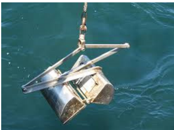
Figure 7 Van veen dredger used for sample collection.
