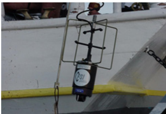
Figure 8 CTD device in the process of descent for data collection.
