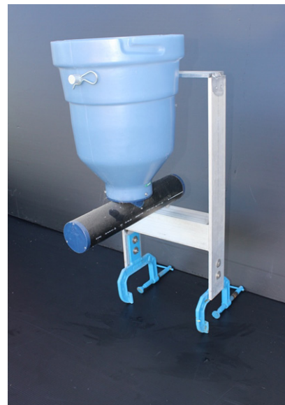
Figure 5 Image of a mount and electric automatic feeder, with the C-clamp tanks used to secure the mount to the side of the fish rearing tank clearly visible.
