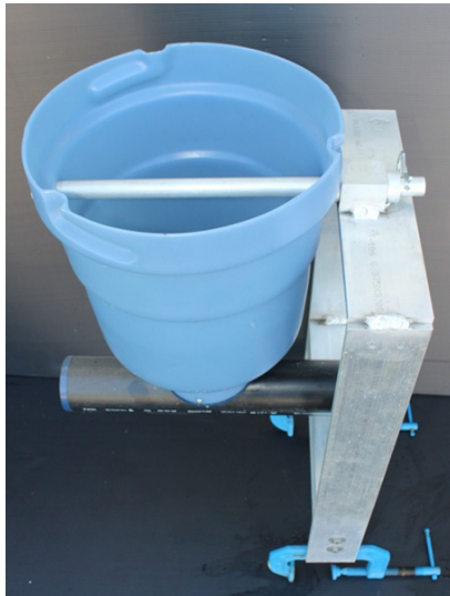
Figure 6 Top view image of a mount and electric automatic feeder.
