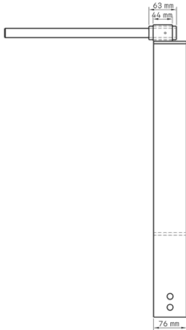
Figure 2 Side view of a mount for an electric automatic feeder.
