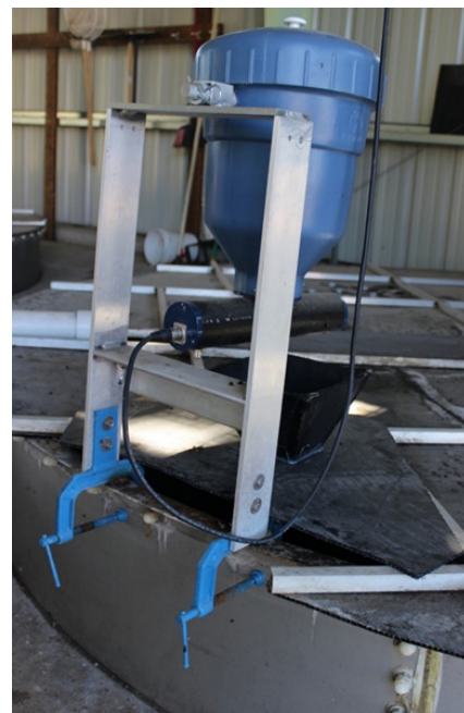
Figure 1 Image of a mount and automatic feeder installed on a 2.7-m diameter partially-in ground circular rearing tank.
