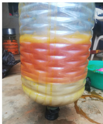
Figure 4 Separation of miscible phases by settling after neutralization: local refining.
