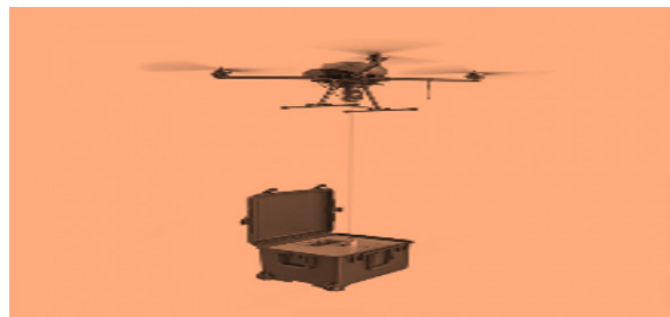
Figure 1 A mobile aviation platform that is “suspended” by taking a sky-dependent flight state connected to the ground mounted on a multicopter base.
