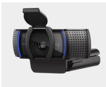
Figure 3 Logitech C920 webcam, used as the low-cost vision system for ArUco marker detection.
