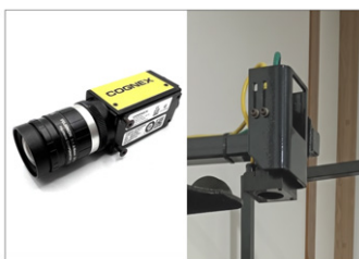
Figure 2 Cognex ISM-1400 industrial camera, configured to detect the target block through native edge and contrast analysis.
