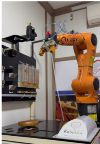
Figure 1 Experimental robotic cell for VGR tests. The KUKA KR6 R900 sixx robot, equipped with a pneumatic gripper, validates the camera's coordinates by manipulating the target block.
