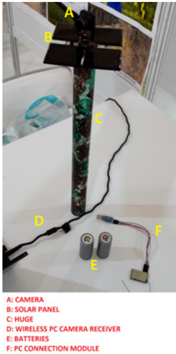
Figure 5 Observation module with radar and camera.
