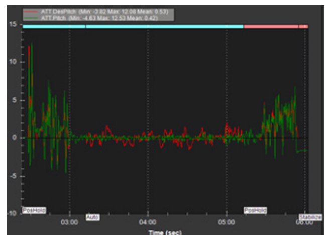
Figure 5 Control of pitch angle in automatic navigation.
