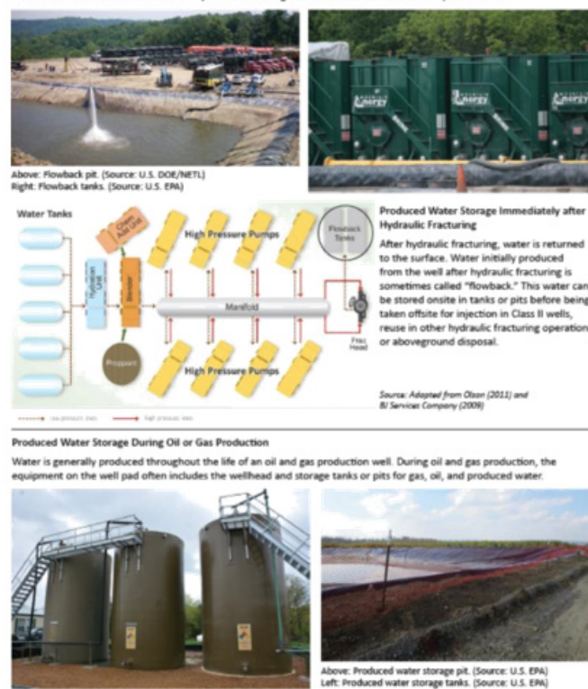
Figure 13 Illustration of storage of flow back water on-site short term (adapted from Olson and BJ Services Company).
