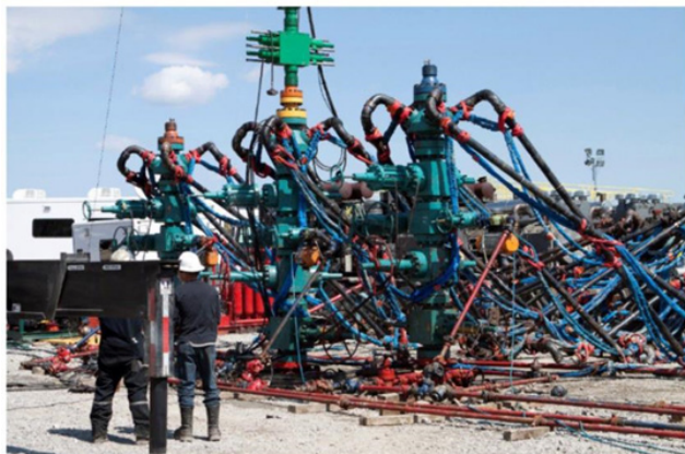
Figure 10 Three wellheads on a multi-well pad connected to the piping used for hydraulic fracturing injection (photo credit: DOE/NETL).
