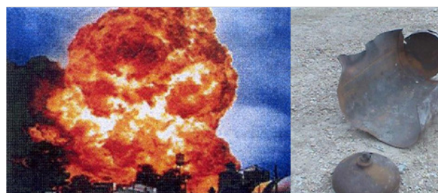
Figure 27 BLEVE from a fireball on a pressure vessel and fragments of the exploded vessel (the time of 1 hour may be much shorter).
