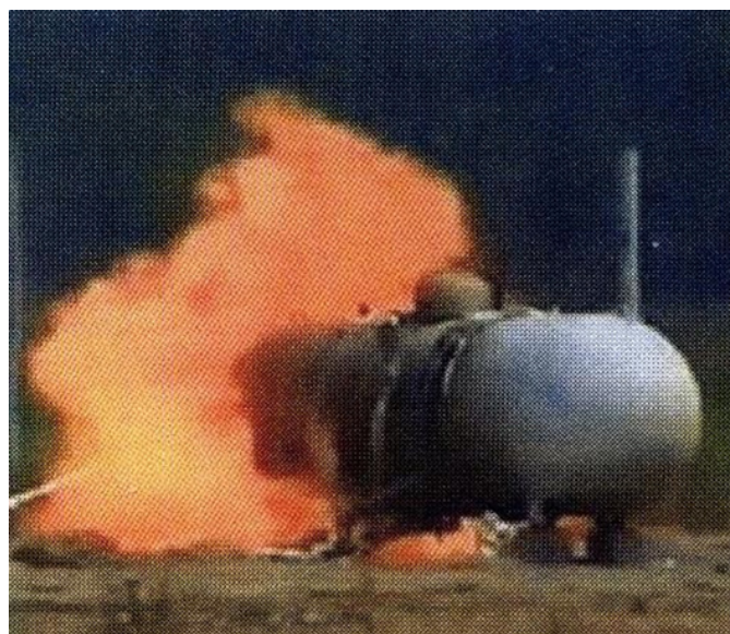
Figure 23 Gas jet flame impinging on separator vessel.
