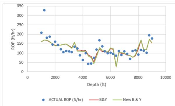
**Figure 2** Actual, initial B&Y and new B&Y ROP vs. well depth.
