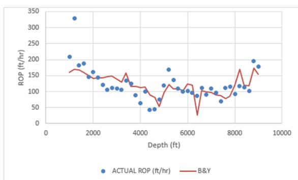
Figure 1 Actual & predicted ROP vs. well depth.
