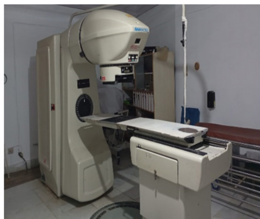
Figure 1 Theratron 780E (1990 model Co-60 unit).
