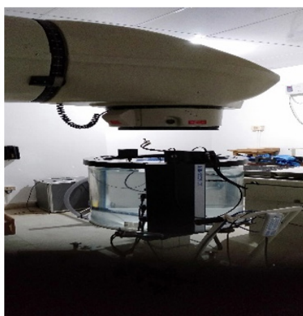
Figure 4 RFA to get beam profiles in 780E.
