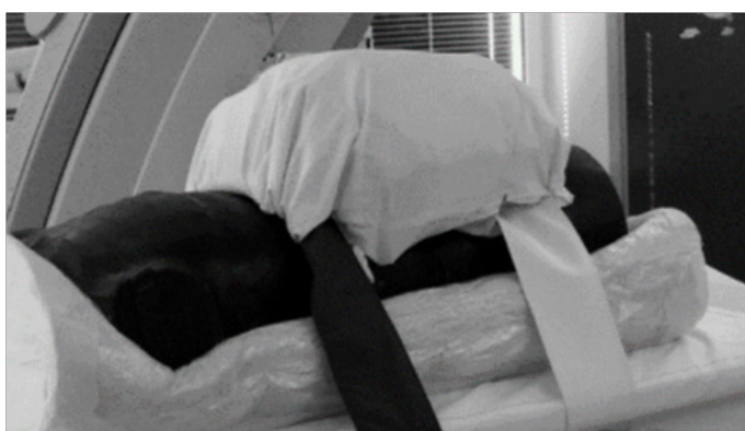
Figure 1 Alderson Rando phantom with sodium bags on top to simulate the third trimester of pregnancy. In the phantom sections 31-35 which corresponds to the uterus, 15 thermoluminescent dosimeters (TLD) were placed to measure radiation dose to the foetus.
