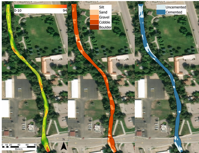
Figure 9 Site 2 bathymetric (left), grain size (center), and cementation (right) maps. Bathymetric chart represents stream depth in cm with contours at an interval of 30 cm.
