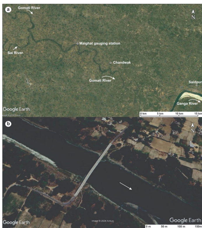
Figure 2 Google Earth images showing (a) distal part of the Gomati River Basin and the confluence of the Gomati River with the Sai and the Ganga Rivers. Gauging station for the Gomati River is located on the left bank at Chandwak and (b) a 100-m wide single sinuous channel of the Gomati River flowing in SE direction at Maighat gauging site.
