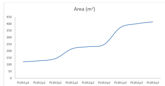
Figure 16 Area of coverage (R) of Pivot sprinkler at various operating pressures.
