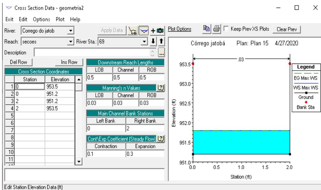
Figure 6 Configuration of section 69 upstream of the channel.
