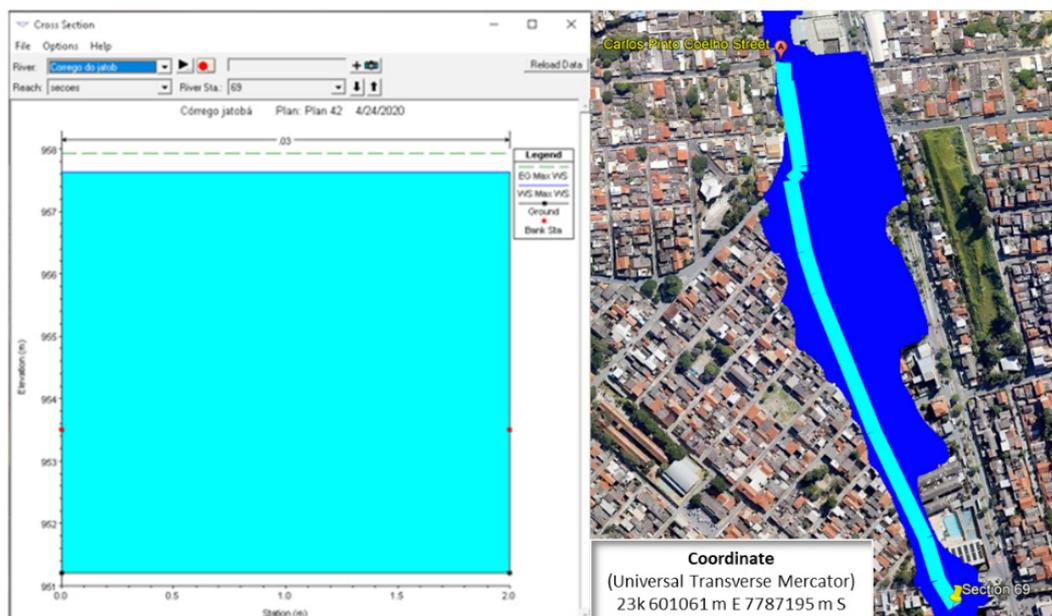
**Figure 7** Overflow of the channel in the face of the worst simulated scenario and its location.
