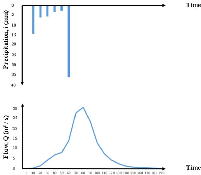
Figure 5 Hyetograph and hydrograph of a 60 minutes rain and 50 years of return period.
