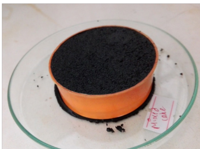
Figure 2 Filter cake prepared from activated charcoal.
