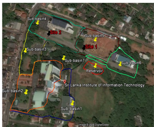
Figure 3(A) Basin area divided into smaller basin area sub basins and identified LID installation.
