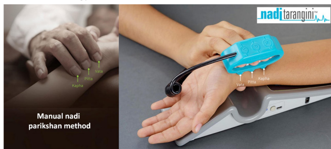
Figure 1 Manual nadi pariksha is done at vata , pitta and kapha locations on the wrist using index, middle and ring fingers respectively. Nadi Tarangini mimics the methodology using three pressure sensors which are used at the three locations to record the nadi data in real time.
