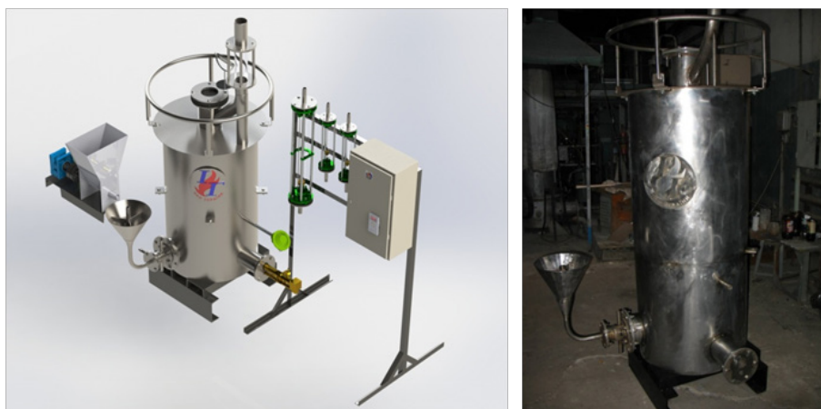
Figure 2 Semi-industrial unit for thermal expanded graphite manufacturing.
