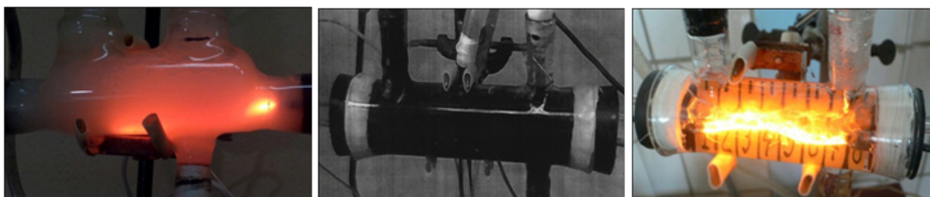
Figure 6 Experimental cell. Research of a critical heat flux at nanofluids boiling.
