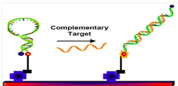
Figure 4 Biosensor model of a chip or slide on which molecular beacon is immobilized.
