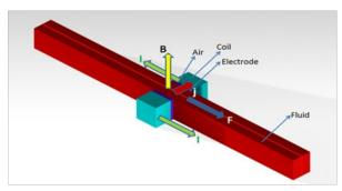
Figure 3 Channel model with electrodes and coils; schematic view.
