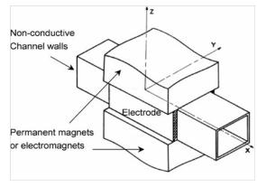
Figure I Schematic view of MHD pumps.
