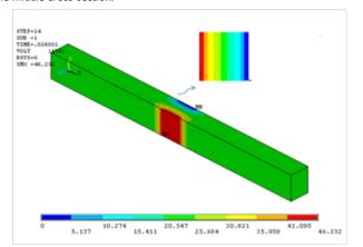
**Figure 7** Potential electric field inside channel and in X=0.0065 m section (edge effects are observable).
