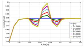
Figure 13 Velocity profile in different electrical field for 3.367 seconds at Y=0.66mm and Z=0.5mm.
