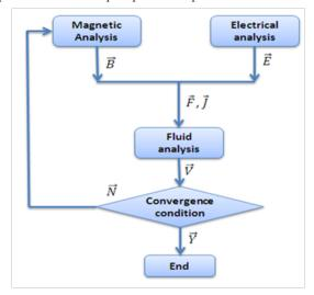
Figure 2 Blood velocity calculation algorithm from the employed electromagnetic fields.
