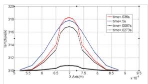
Figure 9 Temperature variation inside channel with applying pulse.
