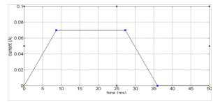
**Figure 5** Considered current graph for electrodes in order to apply fixed electric fields to fluid for temperature calculation (by considering borders impact).
