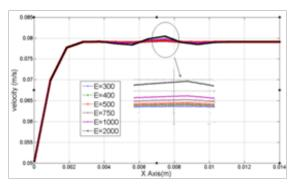
Figure 11 Velocity variation in blood channel for different long-lasting electric fields in range of X=0 to X=14mm with Y=0.666mm & Z=0.5mm.
