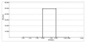
Figure 12 pulse of applied voltage difference to the electrodes.
