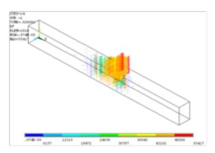
Figure 8 Electrical field distribution inside channel.
