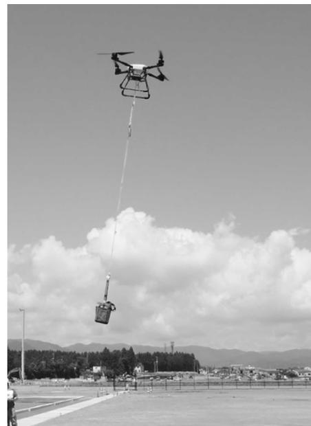
**Figure 1** Unmanned aerial vehicle (UAV) hung and transported the active transport refrigerator (ATR) containing red blood cell solution in the Fukushima Robot Test Field.
