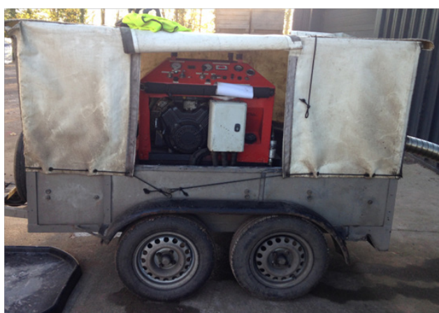
Figure 18 Sam thermal fogging machine used for CIPC thermal fogging in potato (Author's own work, 2017).
