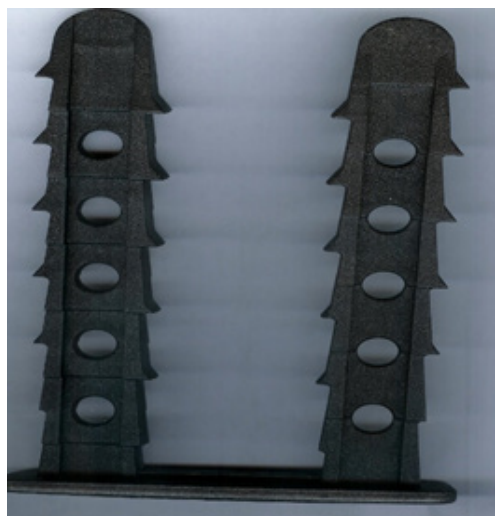
Figure 7 The factorial design of prototype 1 used to anchor the geonets and one per meter net was enough.
