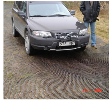
Figure 8 Our project leader surprised after been driving back and forth 10 times on a peatbog with PPnet anchored with what we called prototype 1 and he could just return back to road without any marks after a 2 tonnes car. He stands beside his car just surprised.
