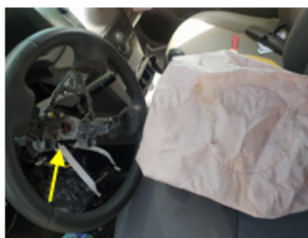
Figure 11 Location of the airbag component inside the steering assembly that matched the fragment removed from the victim in Case 1.
