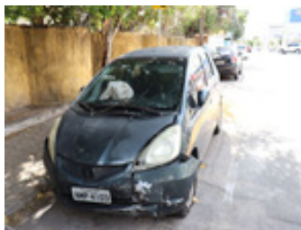
Figure 20 Condition of the vehicle at the time of examination, with emphasis on areas relevant to impact analysis.
