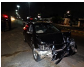
Figure 1 Vehicle from Case 1, showing frontal deformation consistent with a low-to-moderate impact that triggered airbag deployment.
