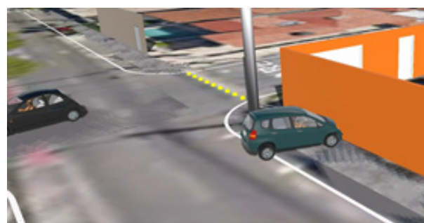
Figure 34 Computer simulation, with a close-up view, of the moment of impact of the Honda vehicle against the wall.
