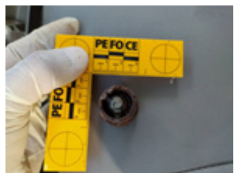
Figure 12 Airbag inflator component recovered from the steering wheel that structurally corresponds to the fragment extracted from the victim's body.
