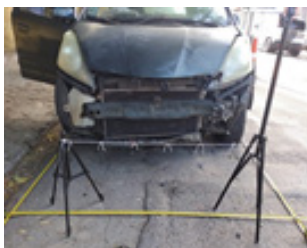
Figure 28 Measurements on the vehicle to estimate speed.
