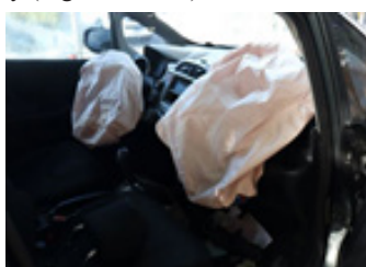
Figure 21 Driver- and passenger-side airbags deployed in the vehicle from Case 2, confirming inflator activation at the time of the collision.
