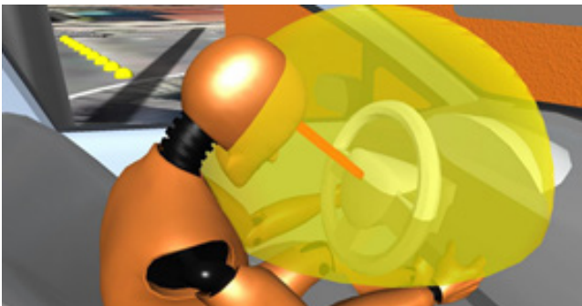
Figure 36 Computer simulation, with a view of the trajectory (in red) of the fragment that hit the victim
