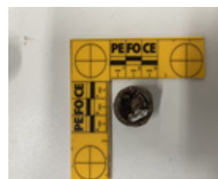
Figure 17 Metallic object removed from the victim's body in Case 2, corresponding to a fragment expelled from the inflator assembly.
