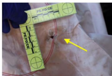
Figure 22 Perforation observed in the airbag cushion from Case 1, demonstrating escape of metallic fragments through the fabric.
