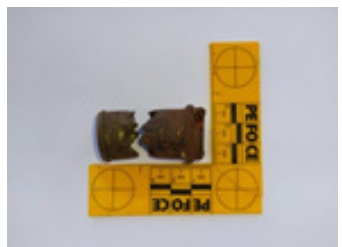
Figure 14 Close-up of the matched fragments, confirming that both originated from the same airbag inflator piece.
