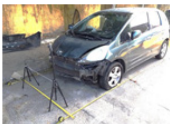
Figure 27 Measurements on the vehicle to estimate speed using the deformation method.
