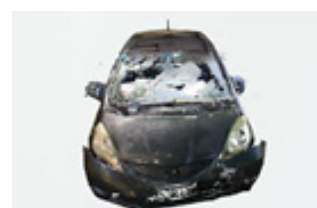
Figure 32 3D model result of the victim's vehicle, after scanning.
