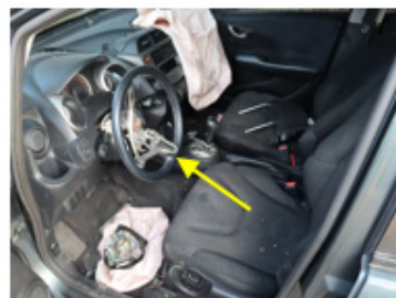
Figure 23 Location within the steering wheel assembly of the airbag component that matched the fragment recovered from the victim in Case 2.
