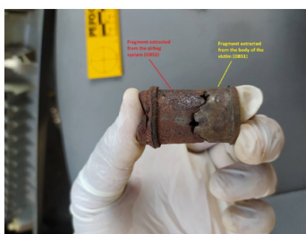
Figure 13 Reconstruction showing the junction of the two fragments forming a single original component from the airbag inflator.
