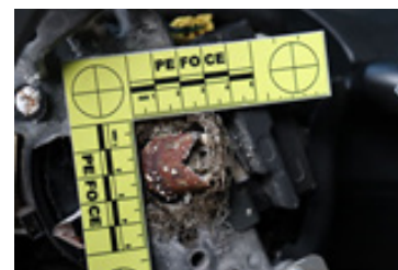
Figure 24 Central steering wheel component corresponding to the fragment removed from the victim's body in Case 2.
