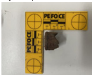
Figure 18 Alternate view of the same metallic fragment removed from the victim in Case 2, showing its deformation pattern.
