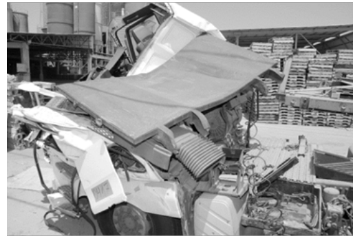
Figure 3 Close-up of the warped wall. Distortions in wall dividing the trailer from the cab.
