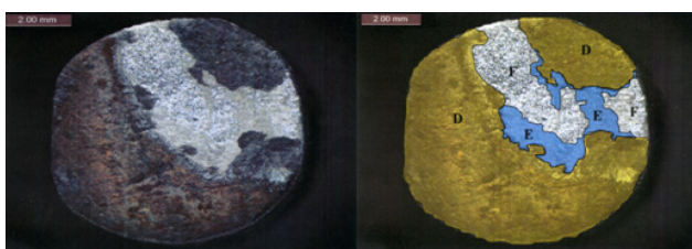
Figure 11 Morphology of a cracked link from the same chain.
