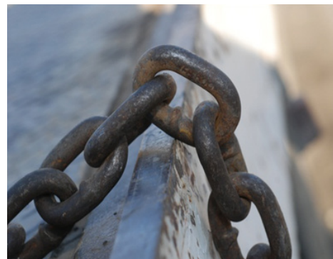
Figure 13 Method of lashing the cargo so that a stress concentration point is created on the chain (simulation).
