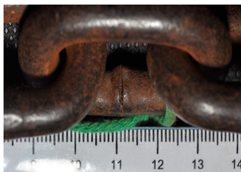
Figure 10 Another cracked link from the chain.
