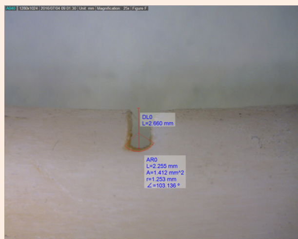
Figure 6: Kerf Floor angle of the Hand Saw.
