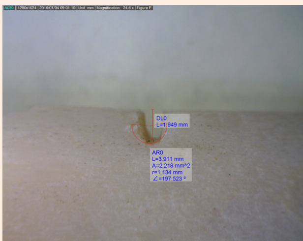
Figure 5: Kerf Floor angle of the Regular Saw.
