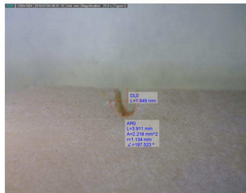
Figure 5 Kerf Floor angle of the Regular Saw.
