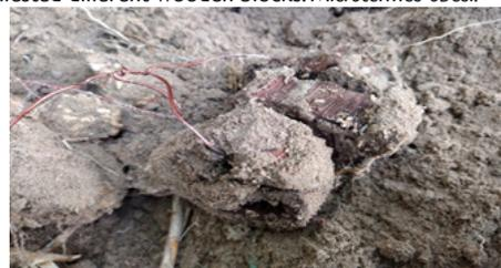
Figure 8 Infested different wooden blocks with *Microtermes Obesi*.
