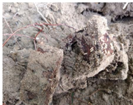
Figure 7 Infested different wooden blocks. *Microtermes obesi*.
