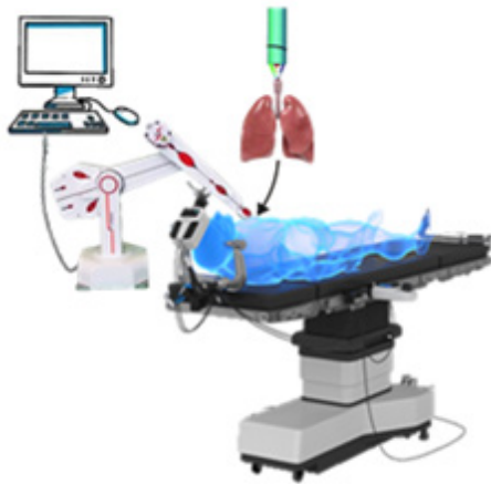
Scheme 1 Diagram of a graphic simplified summary of the notion of robotically assisted in situ 3D bioprinting for less invasive surgery.
