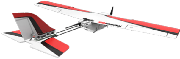
Figure 2 Typical UAV for agricultural use, equipped with visual, multispectral, thermal, hyperspectral and in the near future fluorescence spectrometers to measure Light Induced Fluorescence (LIF), which is very sensitive to many plant physiological processes, their energy metabolism and evapotranspiration.
