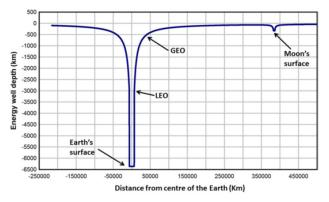
$\ensuremath{\mbox{Figure I}}$  The diagram represents the energy well of the Earth relative to that of the Moon.
