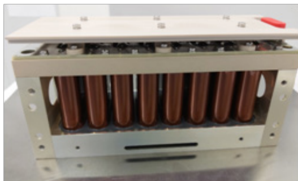
Figure 2 SAB battery single module.
