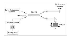
$\begin{tabular}{ll} \textbf{Figure I} A conceptual diagram of Michelson interferometer in OCT system. \\ The resultant interferogram is sent to detector (Copyright Wiley-VCH Verlag to the Copyright Wiley-VCH Verlag$
