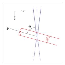
**Figure 3** Coordinate system for blood flow (red) through the optical beam (blue) (reprinted from) (Color online).<sup>19</sup>
