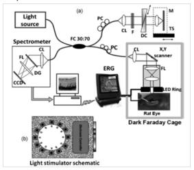
**Figure 2** (A) Conceptual diagram of the combined UHR-OCT and ERG system; here, CL: collimating lenses, DC: dispersion compensation unit, NDF: neutral-density filters, FOI: fiber optic isolator, M: mirror, PC: polarization controllers, TS: translation stage, DG: diffraction grating, FL: focusing lens (reprinted with permissions).<sup>10</sup>
