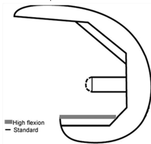
Figure 1 Femoral component of a posterior-stabilized (PS) TKA system: design differences between a standard and a high-flex design.
