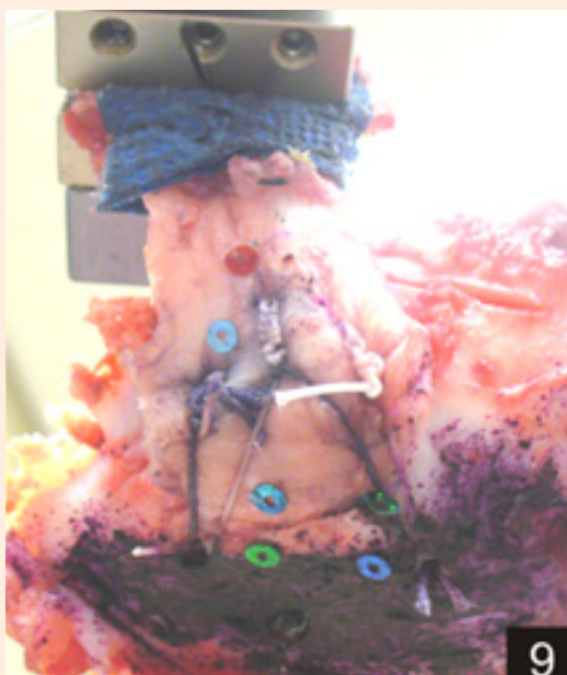
Figure 9: Illustration of the test apparatus with a NTR repaired tendon. Multiple 3 mm markers are positioned on the tendon and bone that are used to determine gap size. Bone lateral to the end of the tendon was stained with Cresyl Violet to aid in gap determination.
