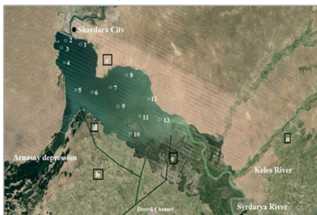
Figure 1 Scheme of sampling stations and sources of pollution in the Shardara reservoir, June 2015: A, B, C—irrigation fields, D—drainage water return that is discharged into the Arnasay Bay, e—water intake from the the Shardara reservoir; 1–13—sampling stations.
