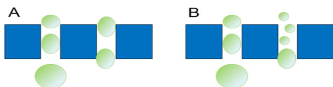
Figure 3 Schematic diagrams of premix membrane emulsification (A) The operating pressure is greater than the critical pressure, (B) The operating pressure is much greater than the critical pressure). 57
