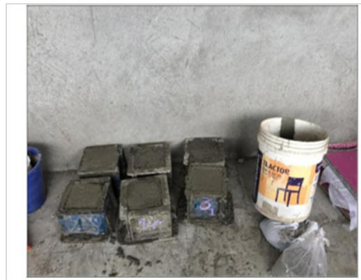
**Figure 4** Grouting mixtures were filling in mould & filled cubes.
