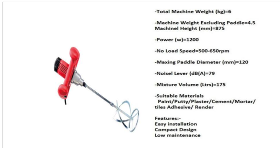
**Figure 1** Shows the mixer and its characteristics.
