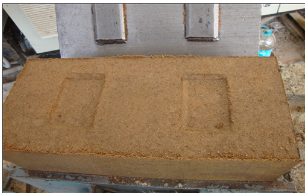
Plate 3 Freshly prepared Compressed Stabilized Earth Block (CSEB) utilizing granite sludge being ejected from the ASTRA machine.
