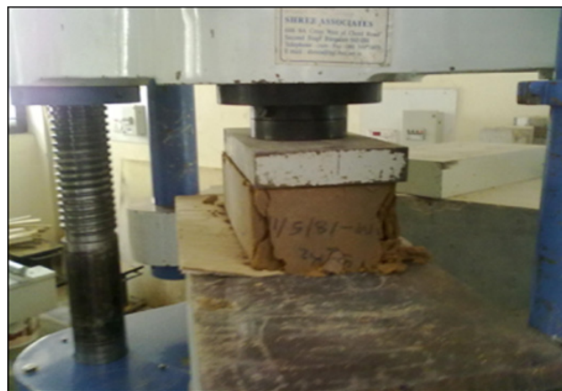
Plate 5 View of wet compression test on CSEB.
