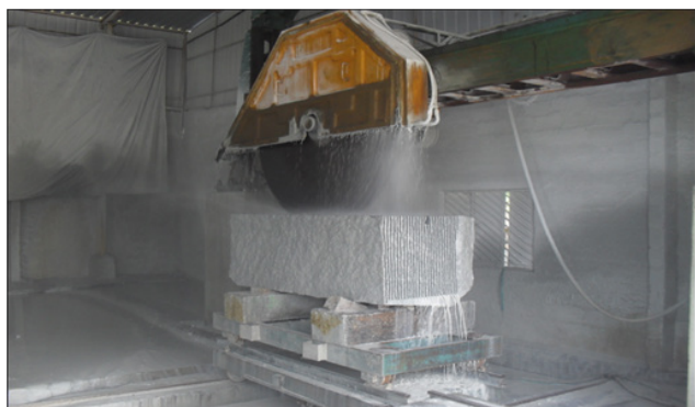
Plate 1 View of granite slurry being formed while slicing granite stone block.
