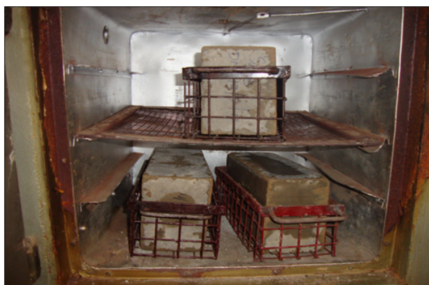
Plate 7 CSEBs placed in wire basket and kept in oven for durability study.
