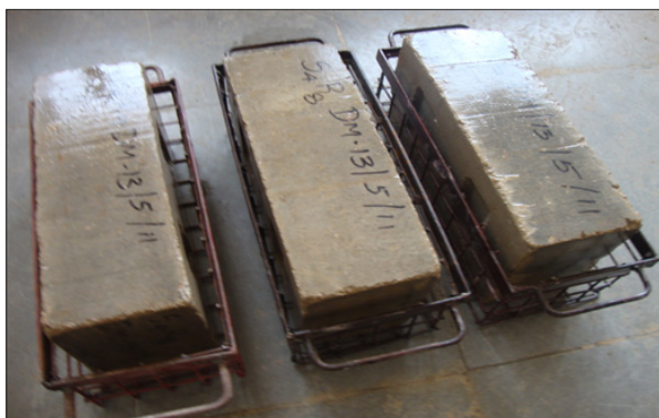
Plate 6 CSEBs being subjected to alternate wetting and drying removed from water and placed in baskets (date of manufacture of blocks can be observed).
