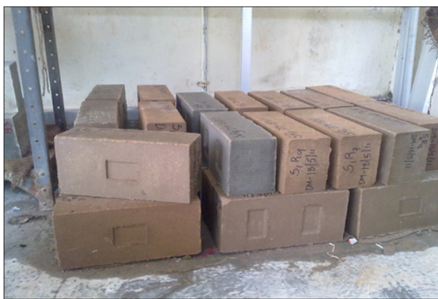
Plate 4 CSEBs of different series stacked for curing.
