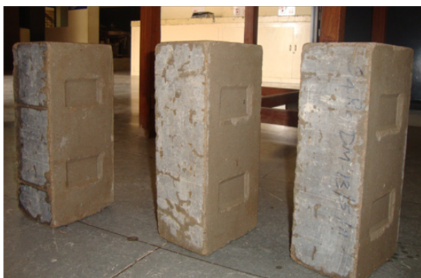
Plate 8 CSEBs after completing 12 cycles of alternate wetting and drying.
