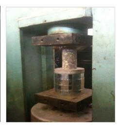
Figure 4 Compressive strength test of core specimens.
