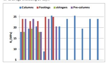
Figure 7 Compressive strength of reinforced concrete elements.
