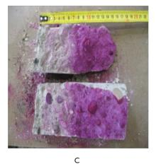
Figure 5 Measurement of hardened concrete carbonation depth.
