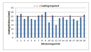
Figure 6 Measurement of the coating thickness of the concrete.
