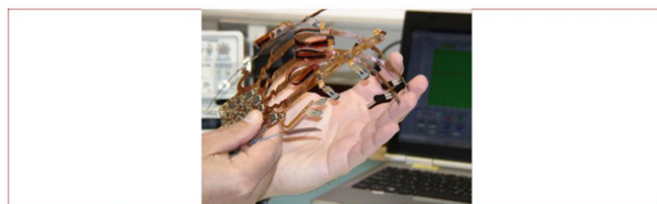
Figure 5 PCB glove under flexion. 14
