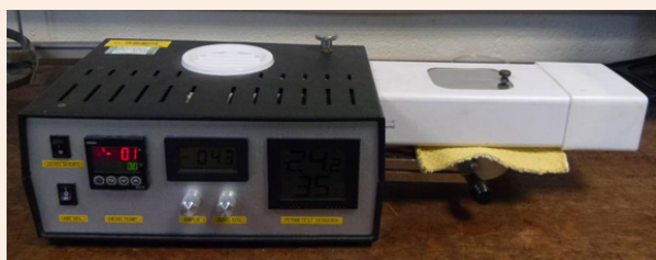
Figure 2: Sensora Permatest water vapour permeability apparatus.
