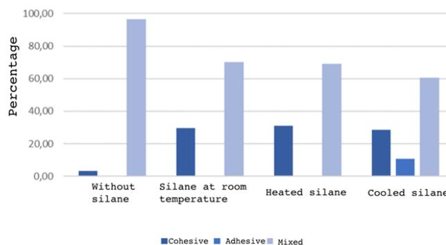
**Figure 2** Frequency distribution for the types of failure according to treatment.
