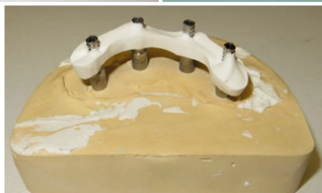
Figures 13–15 Spatial stability tests were carried out on a CST Link® type fiber-reinforced structure, coated with translucent silicone and polymerized on four posts, using a profile projector and doubled with 3D camera measurements: an average deviation of gap of 0.07% (between posts 1 and 3) were observed, which correspond to a gap of 19µm. Plaster control keys, built on a model replica, remained free of fractures and cracks, demonstrating the perfect passivity of the structures.
