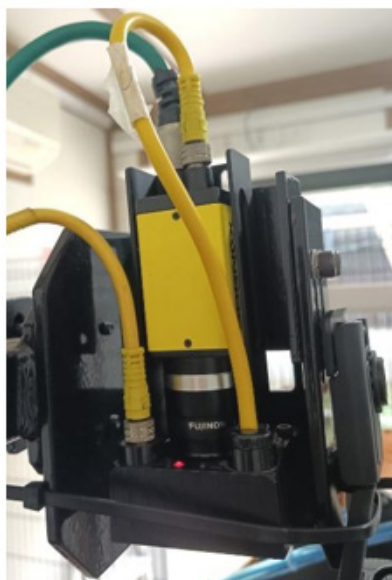
Figure 2 COGNEX camera positioned for inspection.
