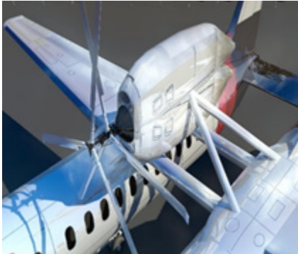
Figure 3 Central rotor hub and engine mount detail.
