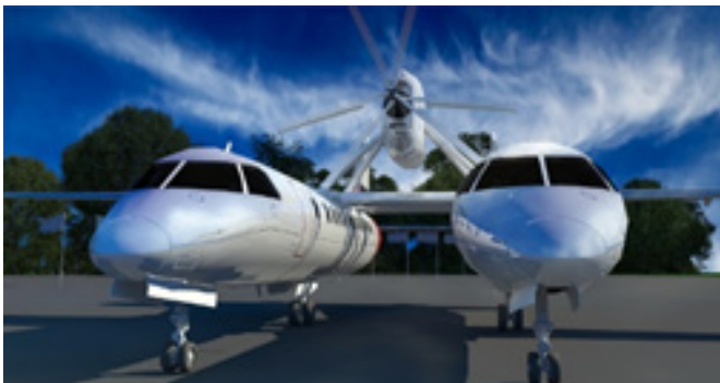
Figure 4 Front view of the twin-fuselage VTOL aircraft in hover mode with helicopter-style rotor control.
