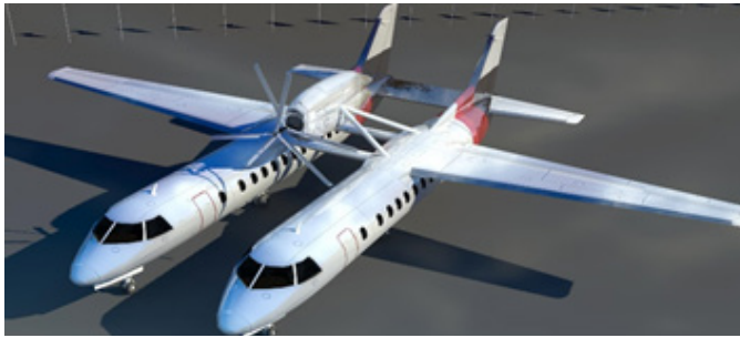
Figure 2 Twin-fuselage VTOL aircraft configuration.
